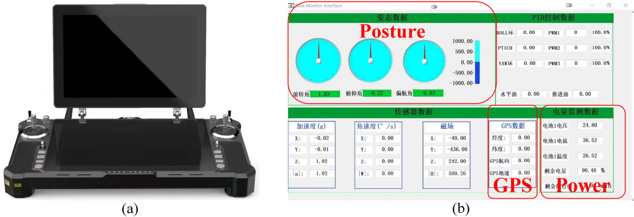
Fig. 17. The handheld ground workstation. a) The appearance of the workstation; b) the monitoring interface of the robot's status.
