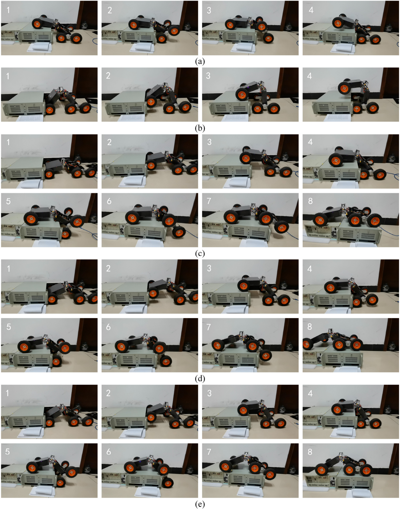
Fig. 20. The experiment of the robot climbing the 200 mm vertical-high obstacle. (a) The robot climbed the obstacle with \delta = 0^\circ ; (b) the robot climbed the obstacle with \delta = 50^\circ ; (c) the robot climbed the obstacle with \delta = 10^\circ ; (d) the robot climbed the obstacle with \delta = 20^\circ ; (e) the robot climbed the obstacle
