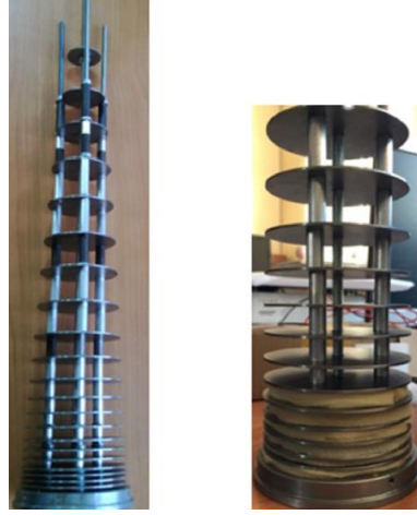
Figure 3.26. Acoustic black hole effect, design SBH-1 of solid discs secured by four steel rods. The left image shows design without any filling, whilst right image contains foam filling between discs. Images presented as from [127].
