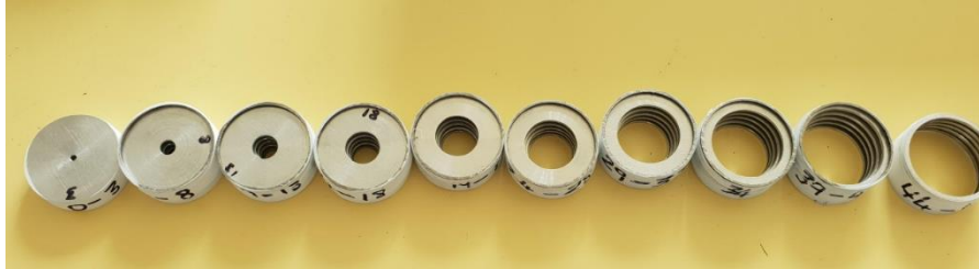
Figure 4.7. Metallic plates for profile absorber building are comprised together in discrete sections with increasing pore diameter.
