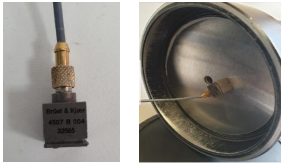
Figure 4.14. Accelerometer measurements performed using Bruel & Kjaer 4507B00433565 and a Bruel & Kjaer impedance tube with standard 2-microphone set-up.
