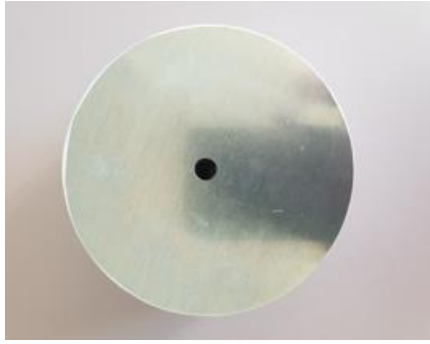
Figure 7.48. Metamaterial pancake absorber front view sealed at the circumference. Dimensions are d_c = 3 mm, d_p = 1 mm, L = 30 mm, r_0 = 4 mm, and R = 50 mm.
