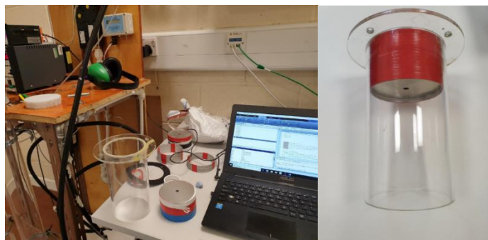
Figure 5.1. Flow rig sample holder and sample segments (left), pancake structure inserted into the sample holder which is then sealed, bolted, and clamped to the flow rig system.
