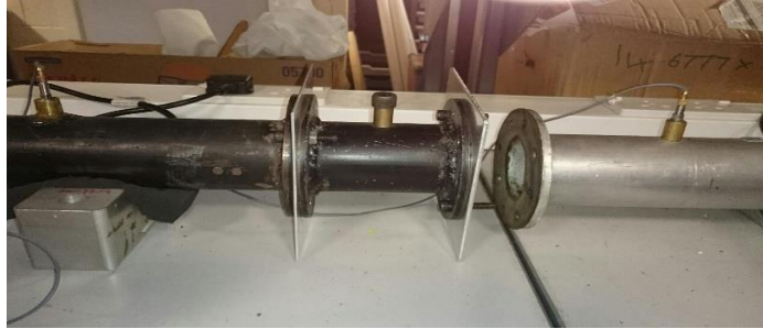
Figure 7.14. Perforated plate tested using the shock tube. The plate had eight pores and tested in rigid backing set up. A cavity depth 100 mm extends the plate followed by a solid end-plate termination.
