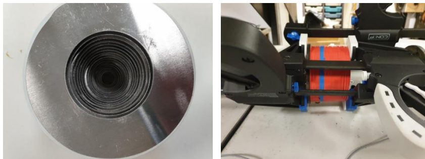
Figure 7.61. Profile structure complete (left) and absorber fixed and clamped ready for shock tube measurements to be performed (right).
