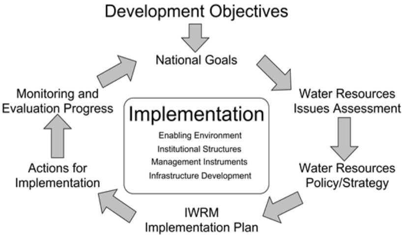
Figure 2.13 Stages in IWRM Planning and Implementation.
