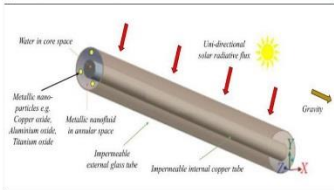
Fig. 1: Geometrical and physical model for annular nanofluid solar collector
