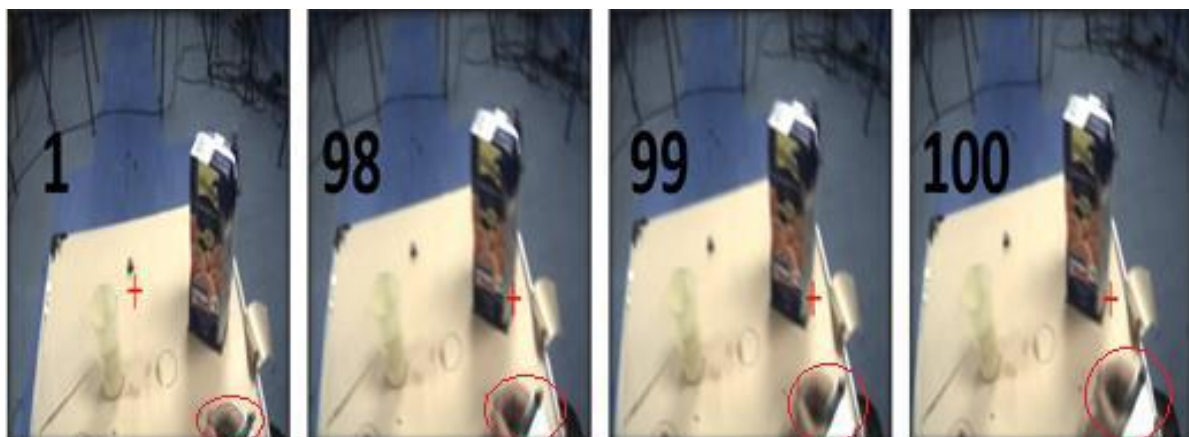
273 274 Figure 4. Example results obtained from the second fuzzy controller demonstrating how the frames 98 and 99 are 275 closer to keyframe 100 than keyframe 1.
