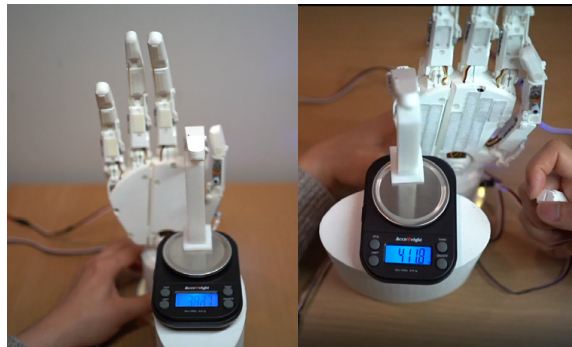
Fig. 9. Electronic scale based fingertip force evaluation.
