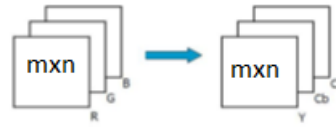
Figure 2. 2 - Colour Space Conversion from RGB to YCbCr. Adapted From (Kuppusamy and Mehala, 2013)
