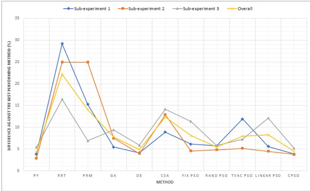
Figure 16: Average performance difference from DA (optimal global path planner) in Sub-Experiments of Experiment II (Execution Time Factor)
