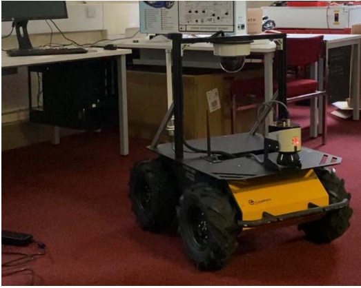
Fig. 1: visualized chassis of Husky UGV showing the mounted LiDAR and the axis network camera
