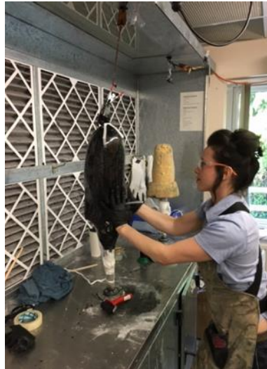
Figure 2-11 Prosthetic socket lamination (Source: Picture taken by thesis author in prosthetics department, DMRC Headley Court)
