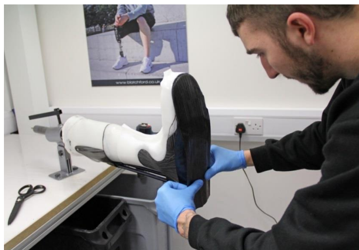
Figure 2-12 Unidirectional carbon fibre being applied onto a PD AFO (Source: picture taken by thesis author at Blatchford manufacturing facility in Sheffield)
