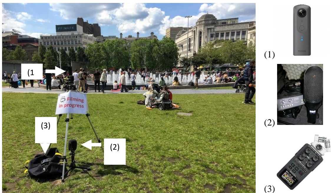
Figure 2 – Equipment setup on field recordings with Ricoh Theta camera (1), Sound field microphone ST250 (2), and ZOOM H6 Handy Recorder (3).
