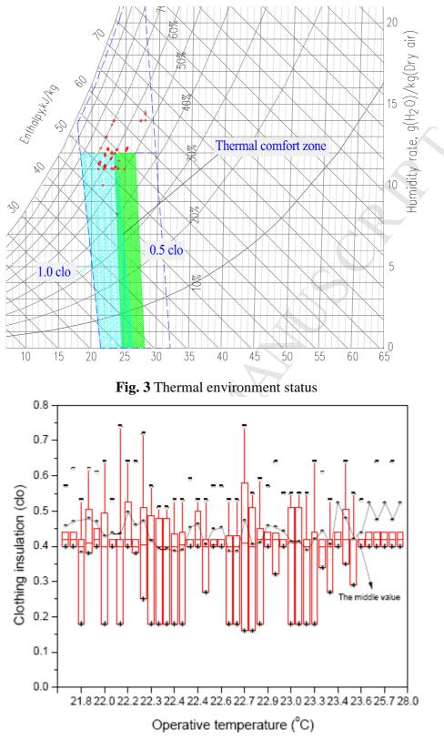
Fig. 4 Variation of clothing insulation with operative temperature
