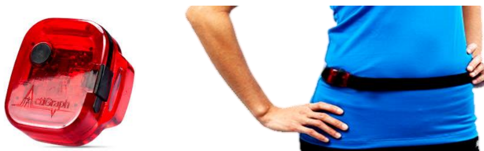
Figure 4.2 Photograph of an ActiGraph GT1M, and a hip-worn ActiGraph attached to a belt (ActiGraph LLC., 2019. [Online]. Available from: www.actigraphcorp.com/actigraph-wgt3x-bt/ )
