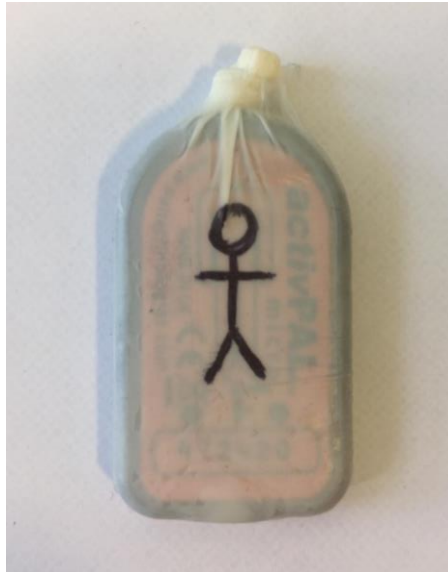
Figure 2.4 activPAL™ in nitrile sleeve and waterproof medical dressing (Author's personal collection)
