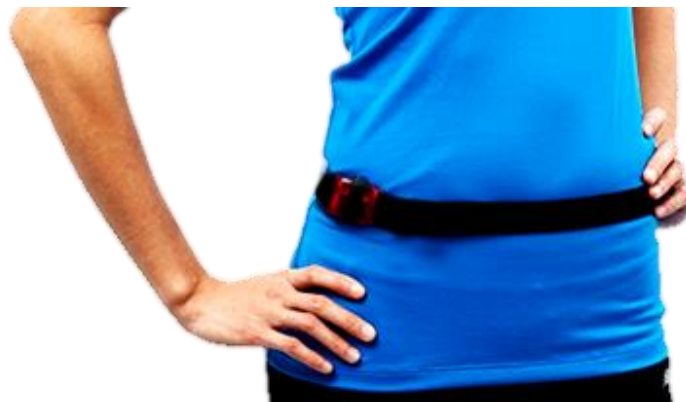
Figure 2.2 Photograph of a hip-worn ActiGraph attached to a belt (ActiGraph LLC., 2019. [Online]. Available from: www.actigraphcorp.com/actigraph-wgt3x-bt/ )
