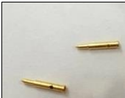
Figure 111. Hollow metallic pin used to hold both antenna tip and the inner conductor of the coaxial cable.
