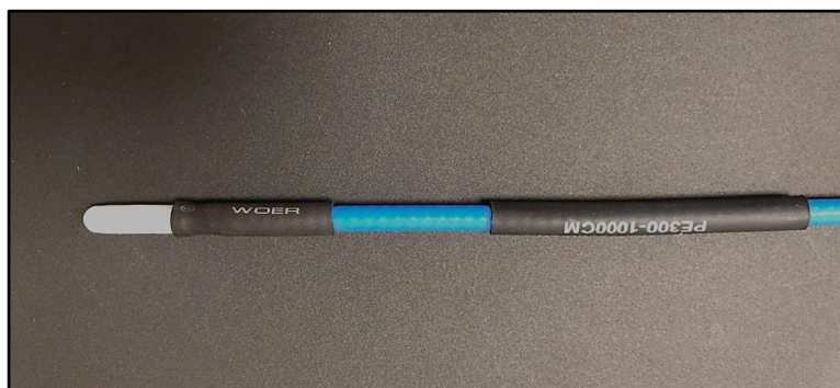
Figure 112. Fully assembled prototype of TDFT applicator connected to the coaxial cable.
