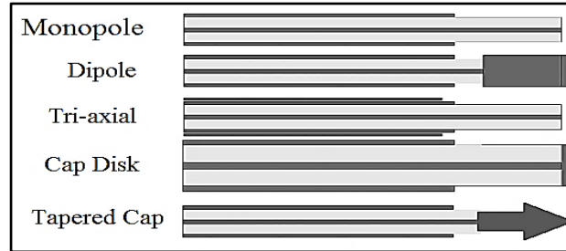
Figure 28. Schematic cross sections of monopole, dipole, tri-axial, Cap Disk and Tapered Cap antenna designs for microwave ablation.
