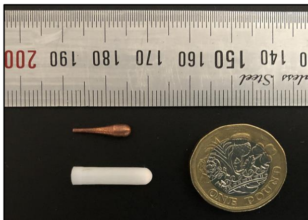
Figure 110. The fabricated prototype of TDFT antenna and its dielectric PFTE shield.
