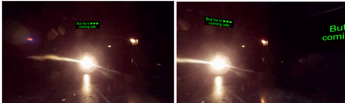
Figure 4: Assistance subtitle with preliminary guiding mechanism that leads to main subtitle and speaker. The subtitle will appear in the current viewing direction at a predefined height and includes a guiding mechanism “arrow” as described below. It will remain at this world-position.
