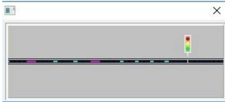
Figure 6.2: Typical screenshot from the new micro-simulation model illustrating vehicles approaching a traffic signal junction
