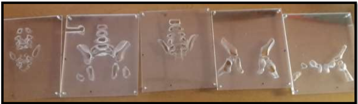
Figure 3. Adjacent PMMA slices, within the PMMA slices are the bony anatomical cavities ready for filling with PoP.
