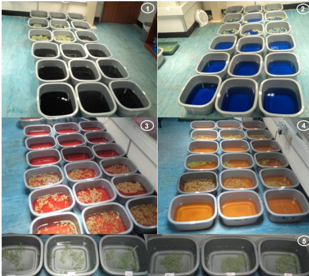
Figure 3.7 Set-up of the second experiment of pond systems. Note: (1), acid blue 113; (2), reactive blue 198; (3), basic red 46; (4), direct orange 46; (5), without dye.
