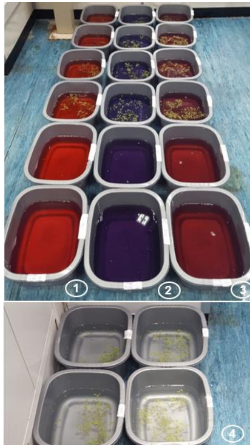
Figure 3.11 Set-up of the fourth experiment of pond systems. Note: (1), mixture 1 (8 mg/l of basic red 46 + 2 mg/l of reactive blue 198); (2), mixture 2 (2 mg/l of basic red 46 + 8 mg/l of reactive blue 198); (3), mixture 3 (5 mg/l of basic red 46 + 5 mg/l of reactive blue 198); (4), without dye.
