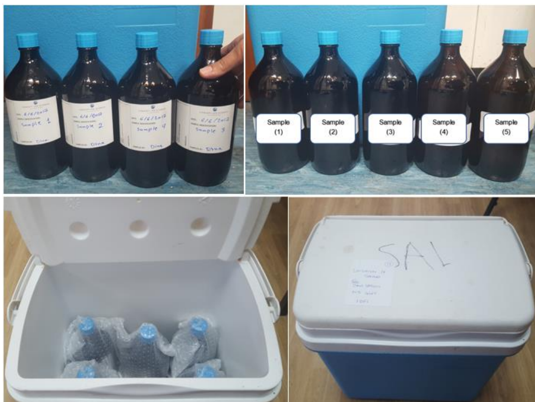
Figure D.4 Outflow samples sent to Concept Life Sciences Analytical & Development Services Limited for GC-MS analysis
