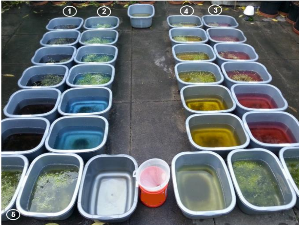
Figure 3.4 Outdoor set-up of the first experiment of pond systems during the third phase. Note: (1), acid blue 113; (2), reactive blue 198; (3), basic red 46; (4), direct orange 46; (5), without dye.
