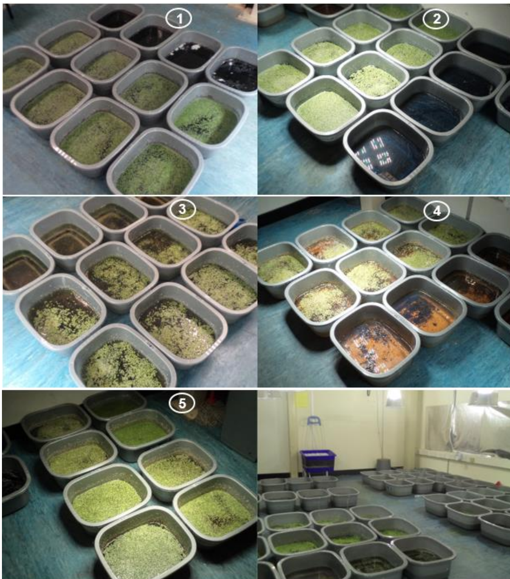
Figure 3.3 Indoor set-up of the first experiment of pond systems during the third phase. Note: (1), acid blue 113; (2), reactive blue 198; (3), basic red 46; (4), direct orange 46; (5), without dye.
