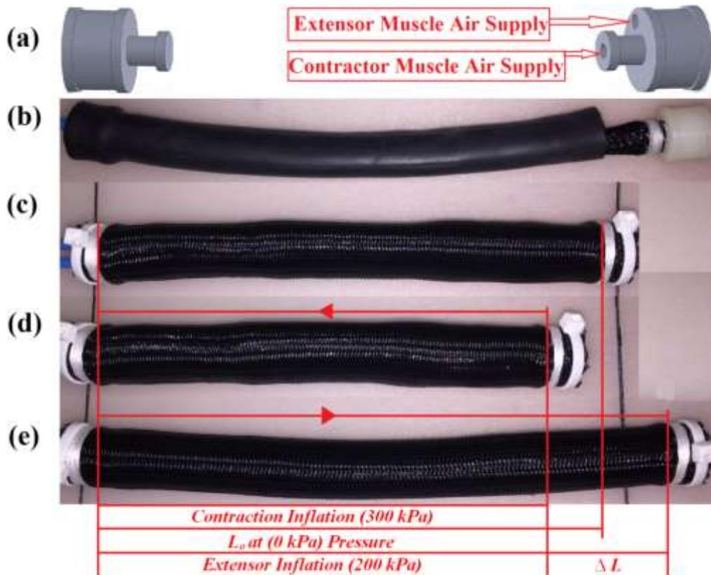
Figure 7. Construction and operation of the novel ECPAM; (a) Endcaps design, (b) The contraction muscle inside the extensor muscle bladder, (c) The ECPAM with no pressure, (d) The ECPAM with pressurised only the inner contraction muscle by 300kPa, and (e) The ECPAM with pressurised only the outer extensor muscle by 200kPa.
