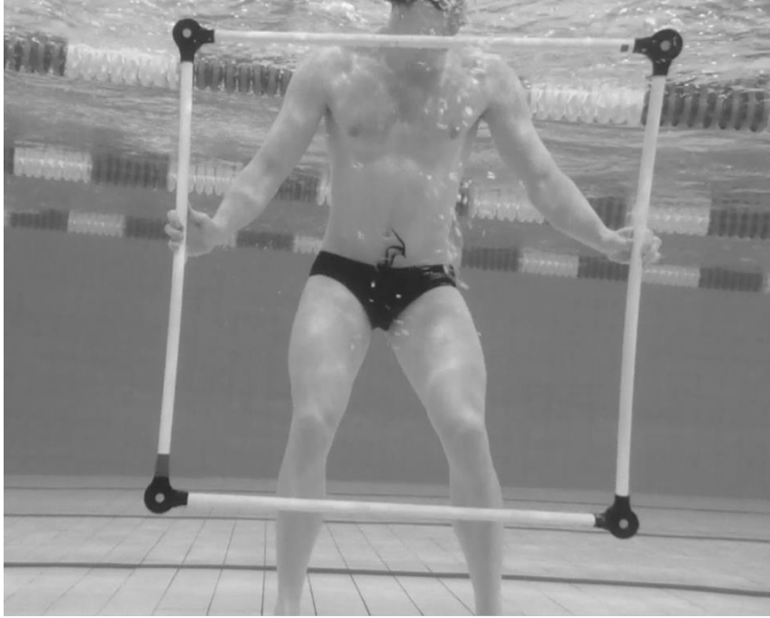
Figure 1 – Picture of calibration square used to measure stroke length.
