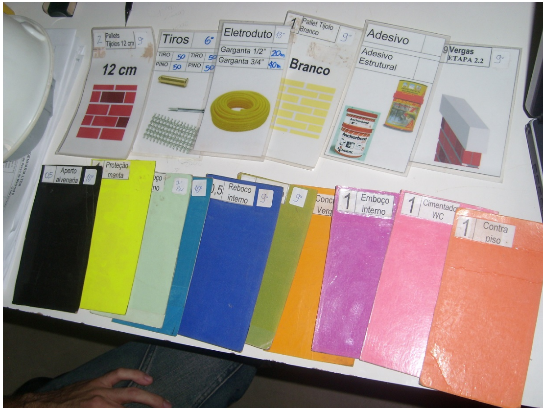
Figure 1. Kanban cards used in construction – the materials shown are pulled by workers from preceding workstations
