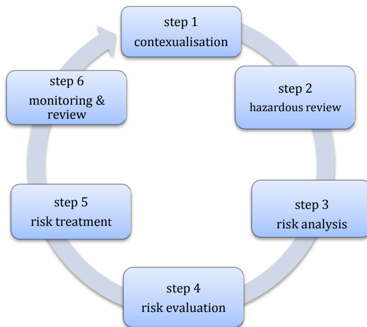
Figure 7. 2: The six-step risk assessment process
