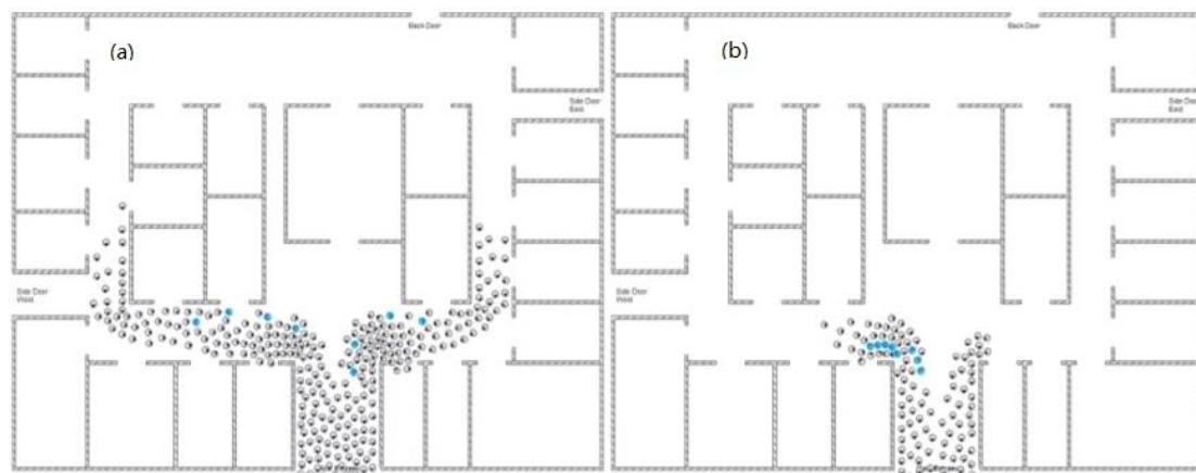
Figure 112 Positions of the elderly people during the evacuation: (a) Case; (b) Case
