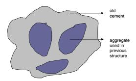
Figure 1. Recycled Aggregate (RA) (Neser, 2006)
