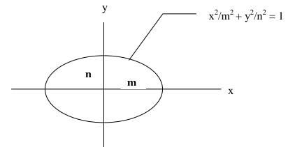
Figure 2 Equation of an ellipse
