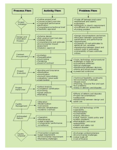
Figure 3: The link between project development process flow, activity flow and problem flow in construction.
