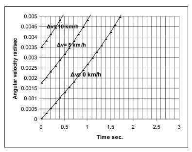
Figure 5. Relationship between angular velocity and time after leader's constant deceleration of -2m/sec2 for different relative speeds
