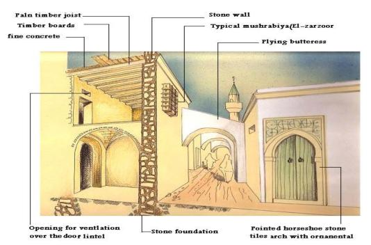
Figure (11) a cross-section of alley and building materials in traditional city of Tripoli : Amer (2007)
