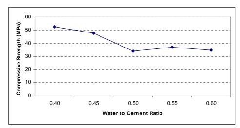
Figure 2. Compressive Strength of RAC at 28 days
