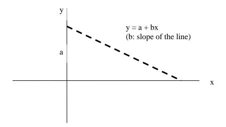
Figure 1 Equation of a line (representing a linear speed-density relationship)
