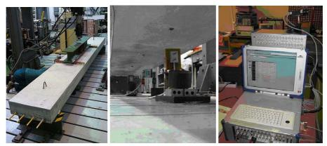
Figure 1. Experimental layout (concrete slab with GFRP - sensors underneath - measuring station)
