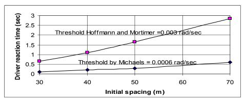
Figure 4. Relationship between driver's reaction time and initial spacing
