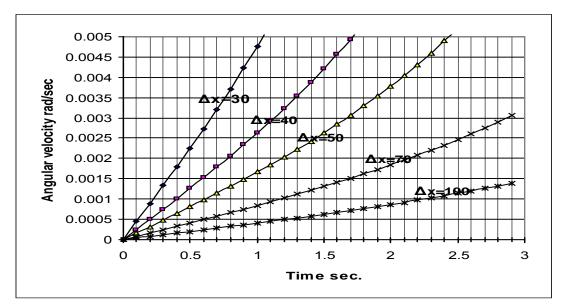
Figure 3. Relationship between angular velocity and time (assuming that leader's constant deceleration is equal to -2m/sec2 for different initial space headways)
