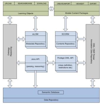
Figure 5: Architecture Framework of the Repository
