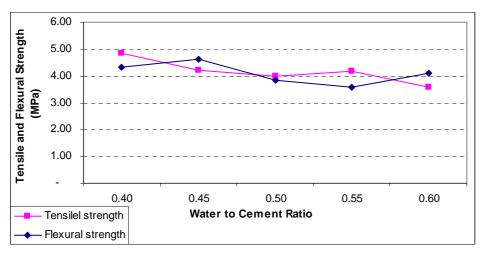
Figure 3. Tensile and Flexural Strength of RAC at 28days
