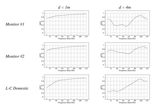
Figure 5 MTFs of 3 Loudspeakers in a Reasonably Well Damped Studio Recording Room at Different Distances d from the Loudspeakers after Equalisation
