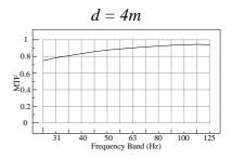
Figure 4 MTFs of a Wide Range Monitor System in a Very Highly Damped Studio Control Room at Different Distances d from the Loudspeaker after Equalisation
