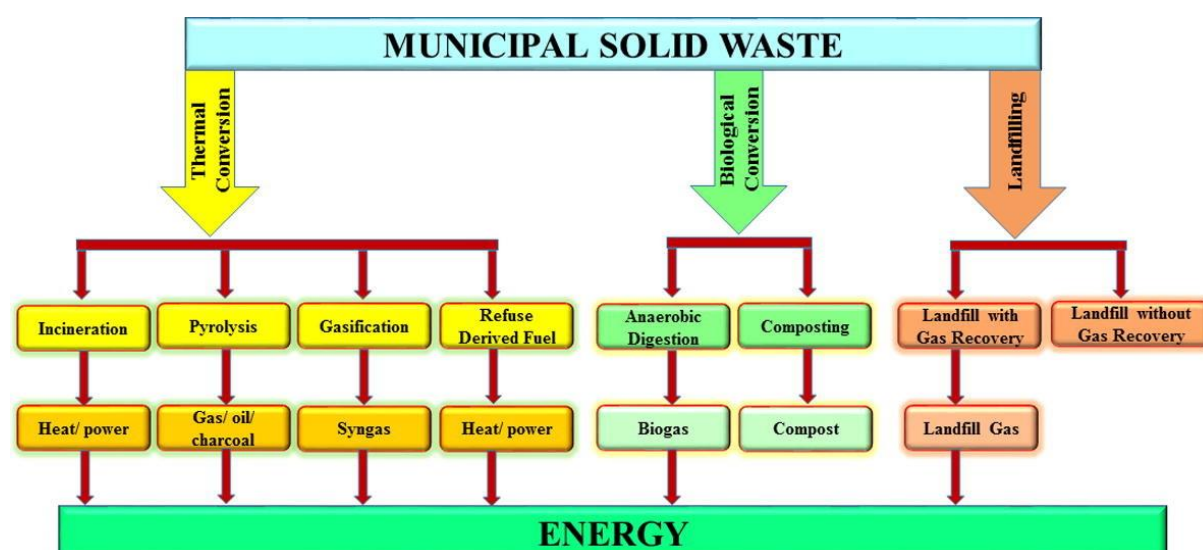
Figure 0.12 Waste to Energy Conversion Categories
